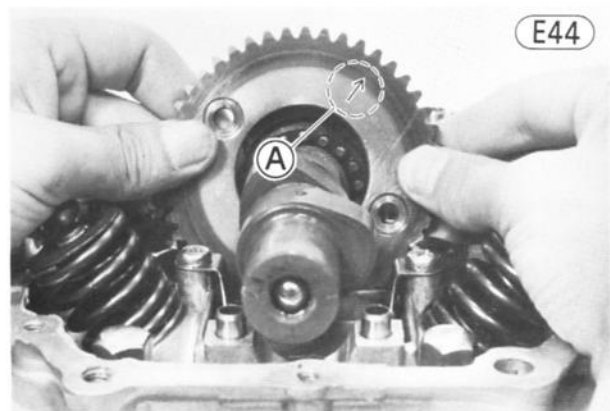
A. Timing Mark (arrow mark)
